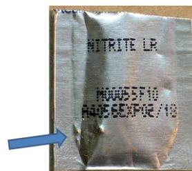
Please tear open the powder pillow and empty the remains into the field test sample cell before performing the colorimeter test.
