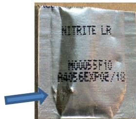
Please tear open the powder pack and empty the remains into the field test sample cell before performing the colorimeter test.
